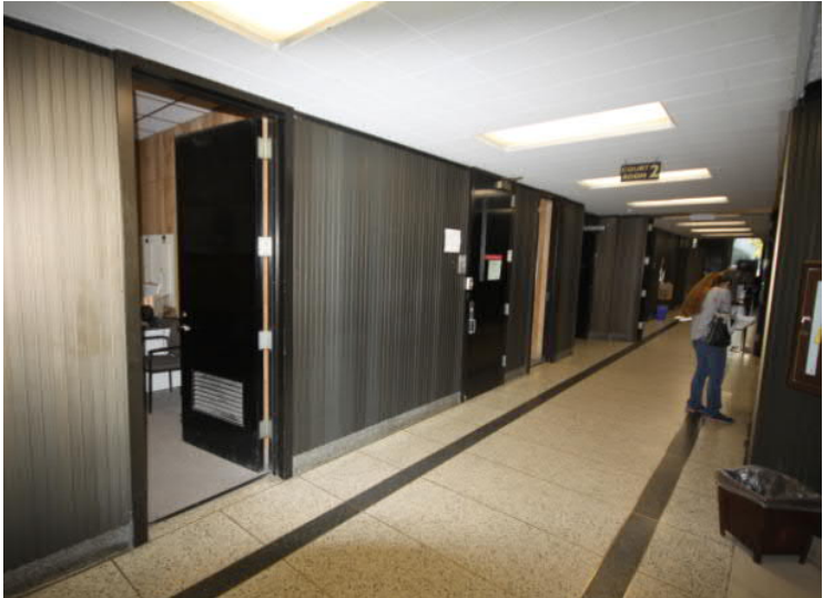
Profiled metal panels, suspended ceilings, and terrazzo tile flooring in the first floor corridor of One Morton Ave.
